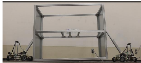
Fig 3. Tilting manipulation for heavy object with 2 mobile robots
