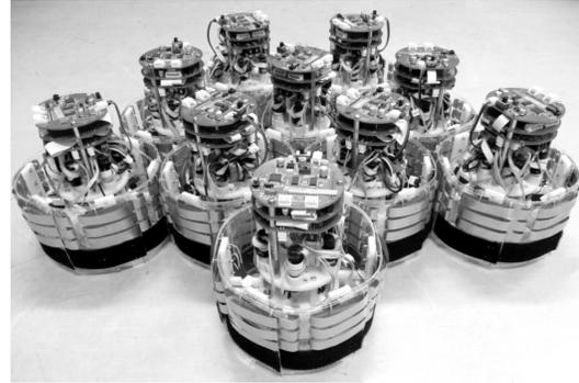
Fig. 1. A real physical Slimebot consisting of 10 modules.
