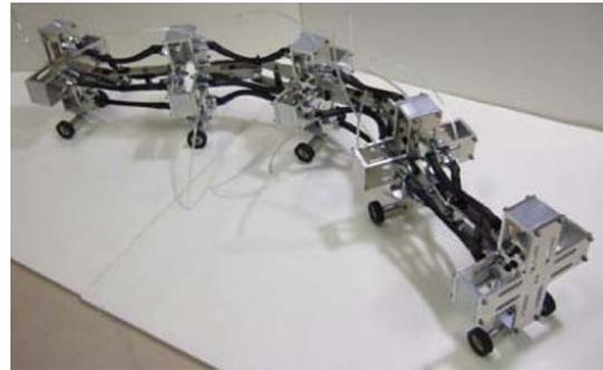
Figure 9: A snake-like robot Pas-1
