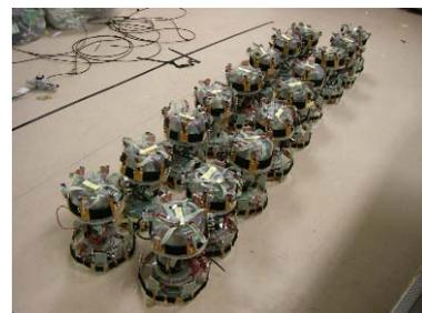
Fig. 8. Modular robot system “Slimebot”
