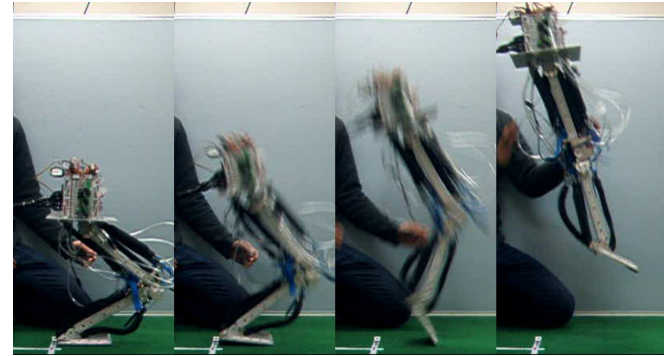
(b) without biarticular muscle activation T_2 = 25[ms], T_8 = 50[ms]
