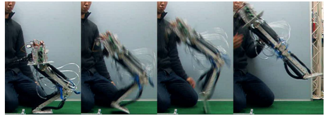
(a) without biarticular muscle activation T_2 = 0, T_8 = 0
