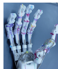
Fig.3 Proposed interference driven finger(a) and wrist(b) based on parallel-wire mechanism. And developed robot hand (c)
