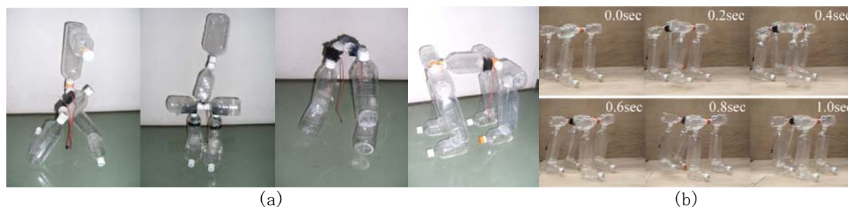
Fig. 2 Plastic-bottle-based robots (a: plastic-bottle-based robots designed by students, b: walking scene of a quadruped robot)
