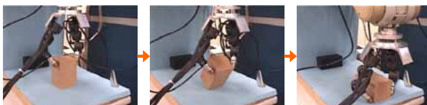
Fig. 4 Execution of Planned Tumbling Operation by Multi-Fingered Hand
