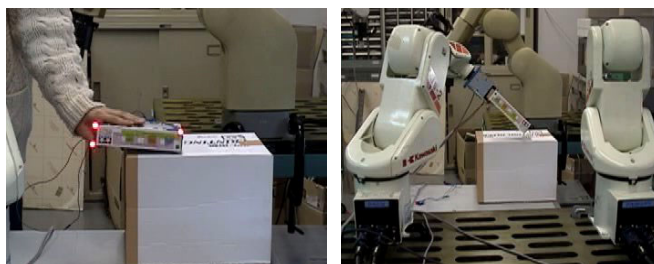
Fig. 4 Human Demonstration of Manipulation and Playback of the Demonstrated Manipulation
