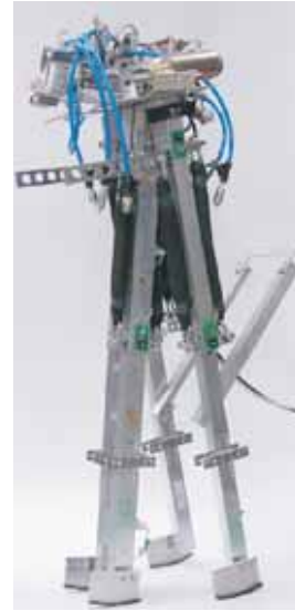
Fig. 1. A biped robot driven by agonistic and antagonistic pneumatic actuators
