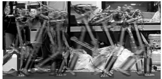
Fig. 6. Running experiment: the flight time and speed were 0.12[s] and 1.13[m/s], respectively. Air pressure was 0.6[MPa]. It could run 5 steps at most.
