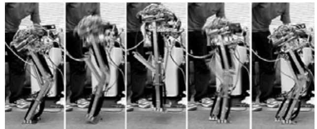
Fig. 5. Jumping experiment: the flight time and height were 270[ms] and 120[mm], respectively. Air pressure was 0.6[MPa]. The robot could jump several times.
